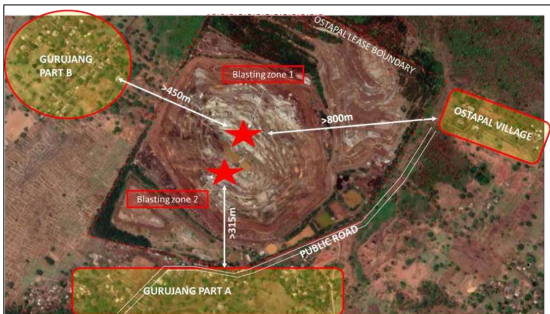
Fig 10: Blasting zones and nearby public/domestic structures
